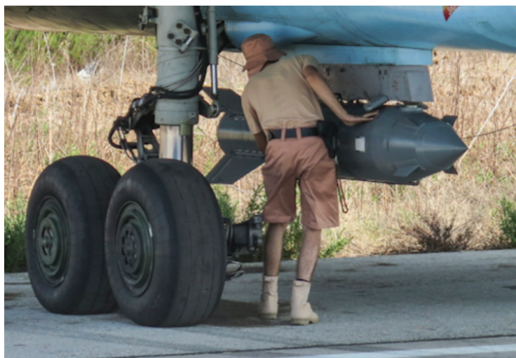
Figure 7: KAB-500S-E being fitted to Su-34 Flanker (2017)
